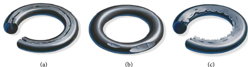
**Figure 1.** Different failure modes of O-rings due to extreme conditions [1] (a) circumferential cracks caused by excessive initial compression; (b) sheared off surface of the O-ring due to faulty assembly; (c) extrusion of the O-ring caused by excessive operating pressure, excessive temperature or too large gap between the shaft and the housing.
