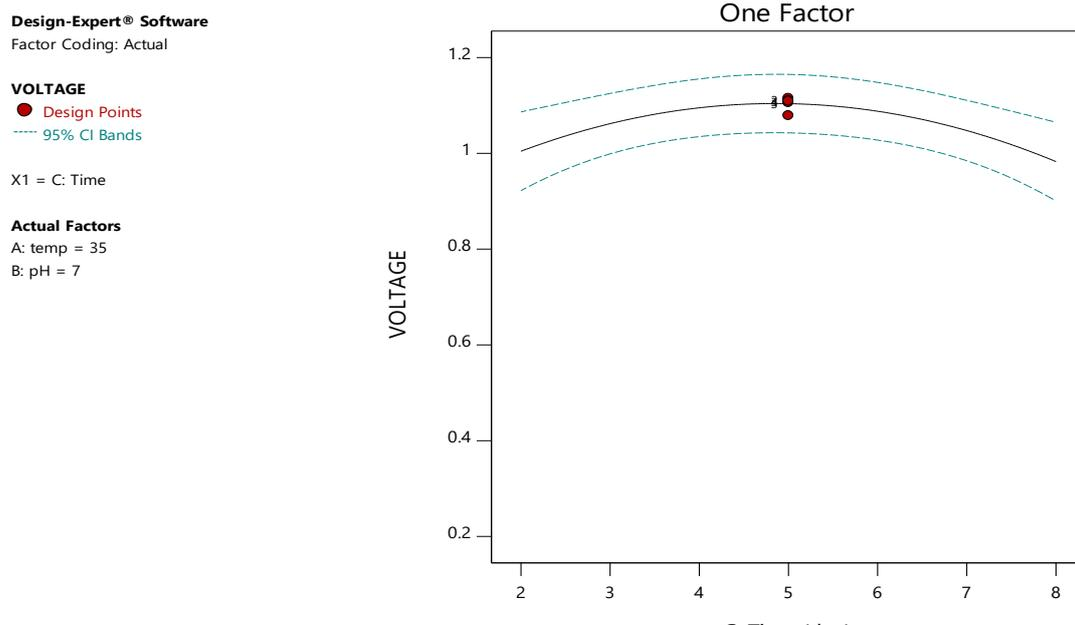
**Fig. 2. Effect of time on the voltage output**
