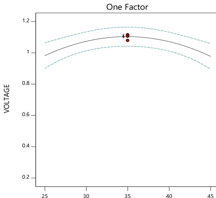
Fig. 4. Effect of temperature on the voltage output
