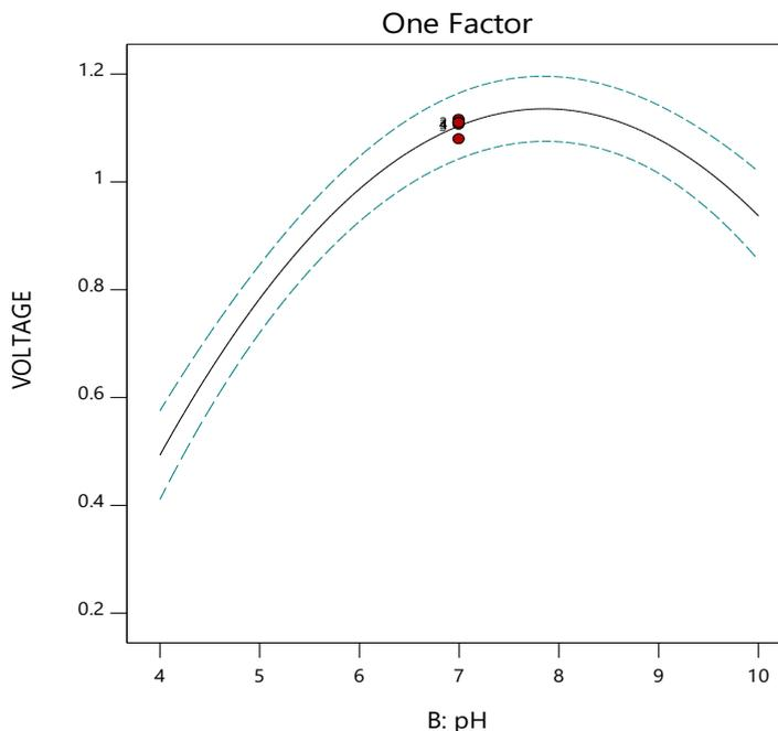
Fig. 3. Effect of pH on the voltage output
