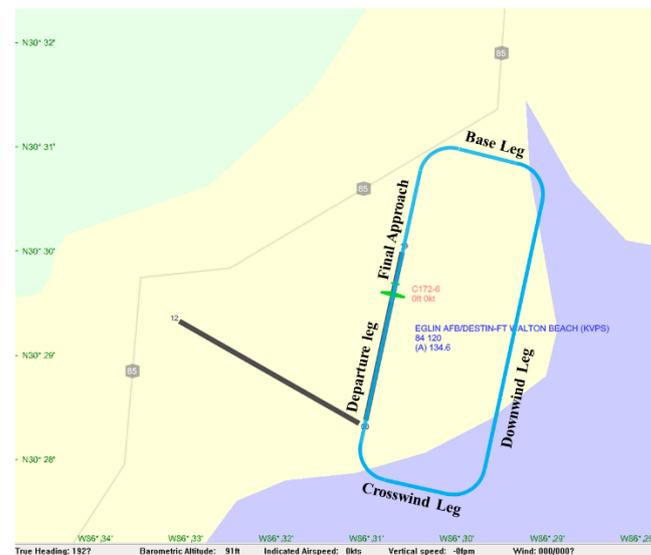
**Figure 5.** Schematic diagram of airfield traffic pattern path.
