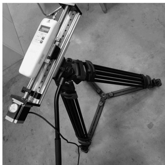
**Figure 5.** Tensile-force measurement system.
