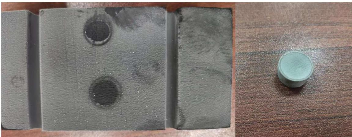
**Figure 11.** Tire sample and sea ice sample after the test (Zhuhai seawater sample,  $-30\text{ }^{\circ}\text{C}$ ).
